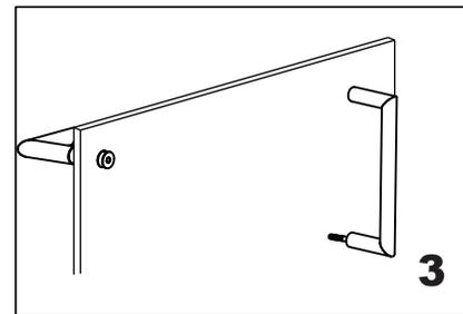
Install the horizontal handle (bolt) through the glass, make sure the set screws holes in the bottom.
