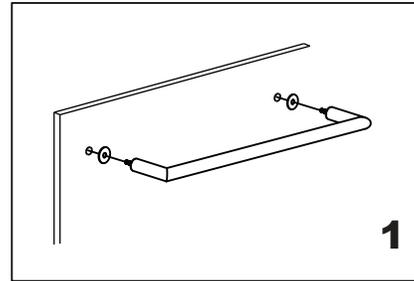
Install the vertical handle (bolt) through the glass holes, make sure the rubber gaskets are between handle & glass.
