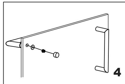
Screw in the bracket onto the bolt, fix the backing (end cap) onto the bracket.
