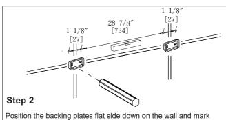
Position the backing plates flat side down on the wall and mark holes with pencil.
