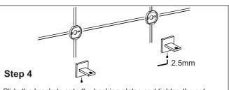
Slide the brackets onto the backing plates and tighten the set screws using Allen key provided.
