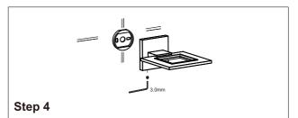
Slide the accessory onto the backing plate and tighten the set screw using Allen key provided.
