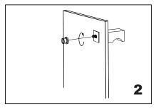
Screw in the fixing bracket into the knob bolt.
