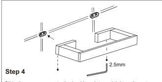
Slide the accessory onto the backing plate and tighten the set screw using Allen key provided.
