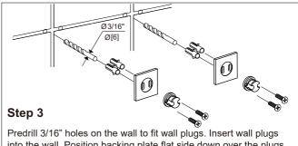
Predriil 3/16" holes on the wall to fit wall plugs. Insert wall plugs into the wall. Position backing plate flat side down over the plugs and install screws.
