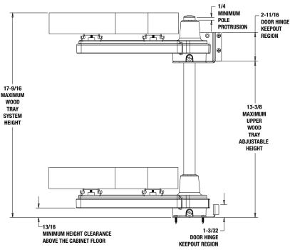
Using the diagram as a guide, determine the desired height position of the upper shelf and make a light pencil market on the side of the face-frame.
