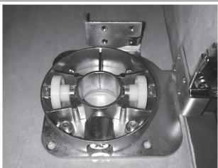
Place the Lower Hub Assembly tight against the back corner of the face frame (the panel divider in frameless applications) and firmly secure with 4 four #8 X 3/4" Pan Head Phillips Wood screws provided as shown above.
