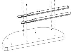
NOTE: The Half Moon Lazy Susan ships ready to install as a Left Hand model. Apply first set of screws on A,B or C when converting to Right Hand model. Attach second set of screws where they are positioned.
