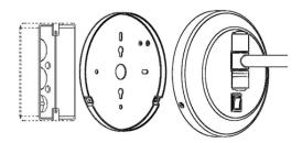
6. Replace mirror base over mounting base plate and secure using the three (3) mounting Hex screws. Restore power to the site and turn mirror fixture on at power switch on base.
