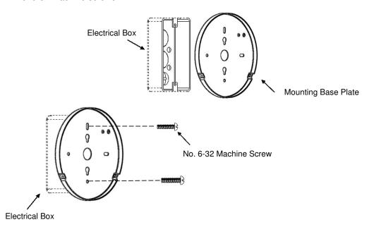
\*\*Note: Sequence of mirror mounting parts with components per UL standard 1598\*\*
